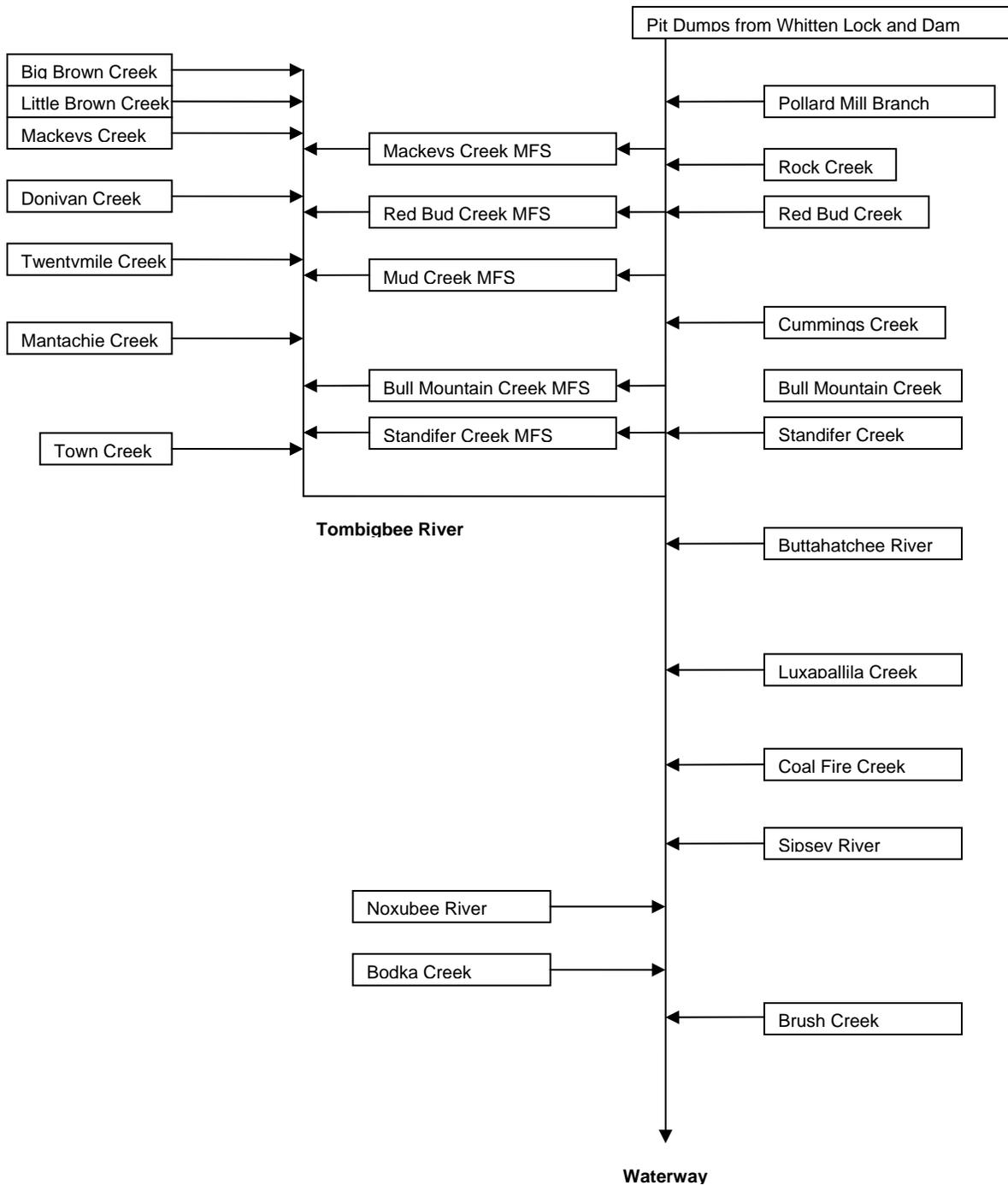
Figure D. Tombigbee River and Upper Tenn-Tom Waterway Flow Chart. (MFS= Minimum Flow Structure)
